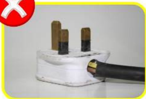
Frayed leads or exposed internal wires are fire risks
